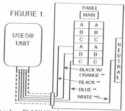
\*\* Conductor colors: BLACK W/ORANGE stripes, BLACK and RED. BLACK W/ORANGE stripe conductor must be connected to the panel's high leg.
