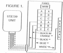
\*\* Conductor colors: BLACK W/ORANGE stripes, BLACK and RED. BLACK W/ORANGE stripe conductor must be connected to the panel's high leg.
