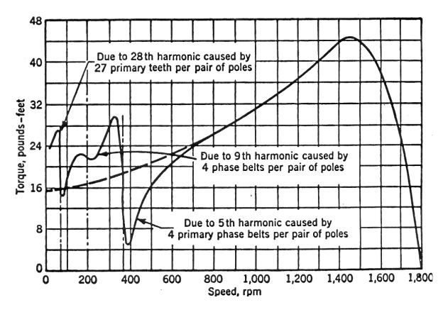
Figure-5 Asynchronous Crawling of Induction Motor
