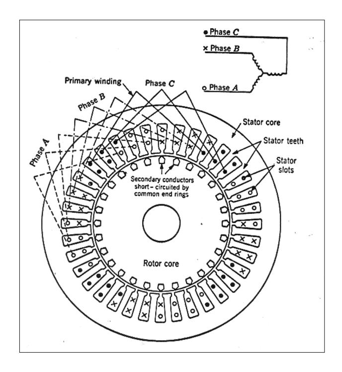
Figure-1 Cross-Section of Typical Three-Phase Induction Motor
