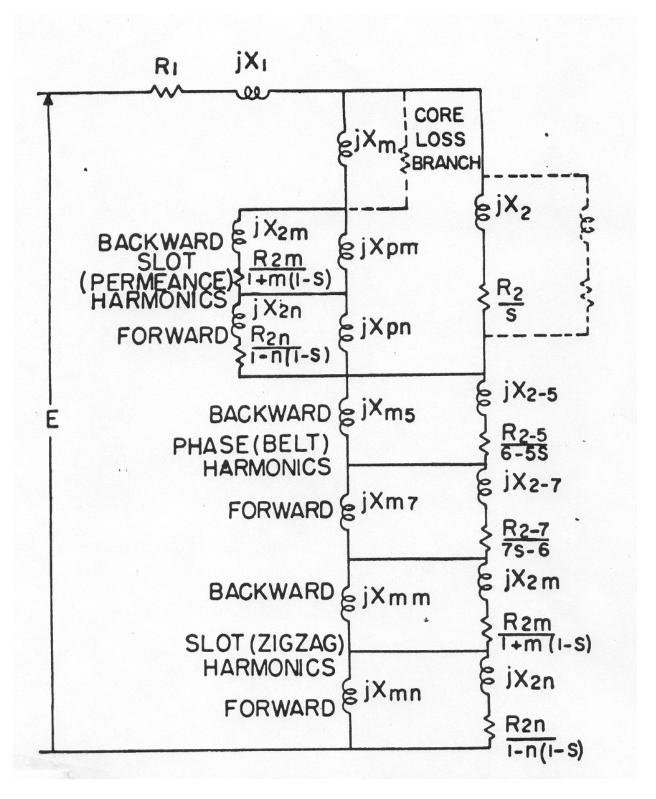
Figure-3 General Equivalent Circuit of a Polyphase Induction Motor
