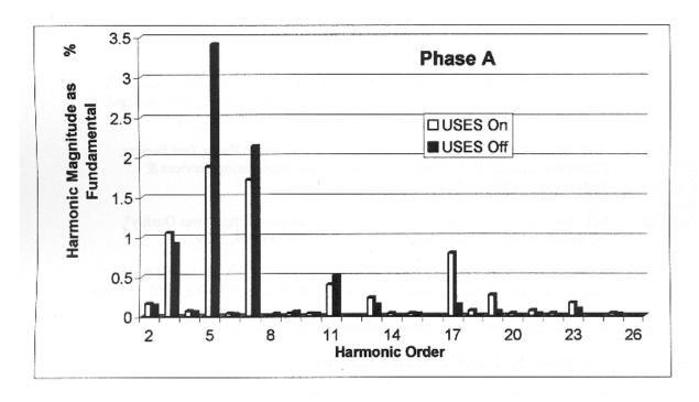
Figure-6. Motor Harmonics for Phase A at 75 RLA with USES on/off.
